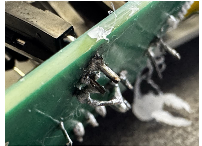
4 Faulty solder joints, redone
