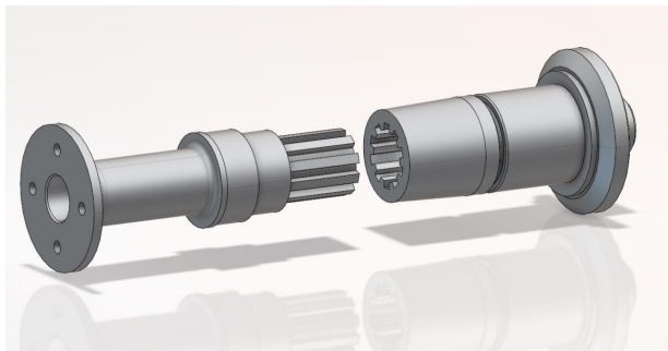
Output shaft in two parts, splined, as the brief required.
