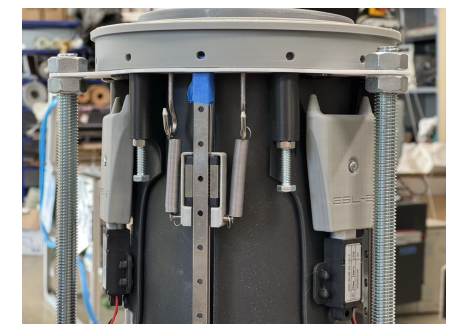
Linear rail and carriage, springs, electric linear actuators and 3D printed mounts.
