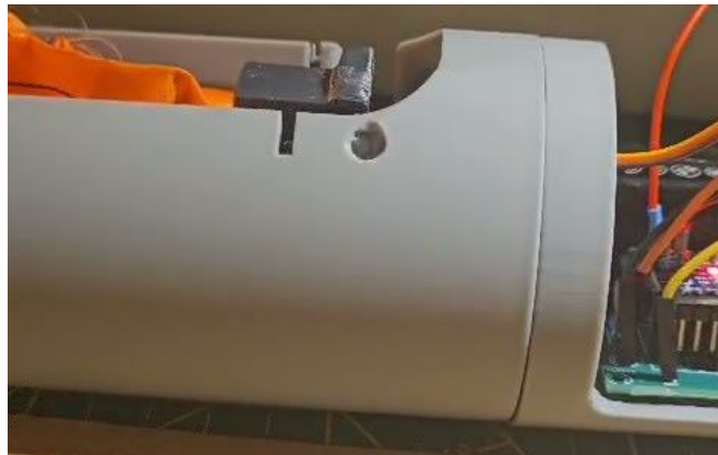
Parachute hatch and its servo latch, bench test, June 2025.
